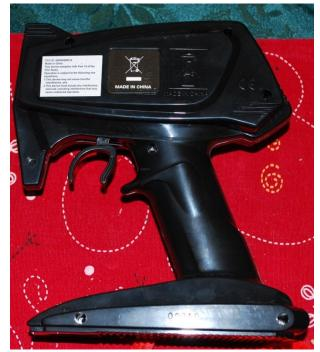
3) Remove the cover from the controller (May have to slice the stickers in the battery compartment of the controller).
